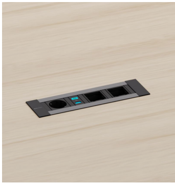
Electrification Box - AC071 267,75x78,6mm support / 258,8x67mm cut out. Surface electrical unit with 1 schuko + 1 USB charge A et C + 2 RJ45 + 1 HDMI. White or black colour.
