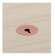
Top Access Round - AC072 Ø140mm support / Ø102mm cut out / Ø80mm passage. Round metal top access with removable cover. Customisable colour.
